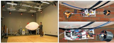
Fig. 7. The left image shows the blimp used in test environment equipped with a motion capture system. It has a customized gondola (right images) that includes an X Scale based computer with sensors, two ducted fans that can be rotated by 360 degrees, and a webcam [15].
