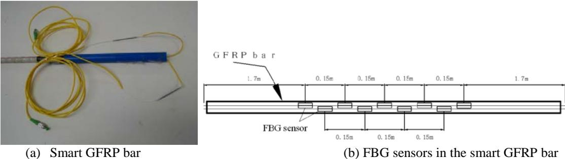
Figure 8 A smart GFRP bar
