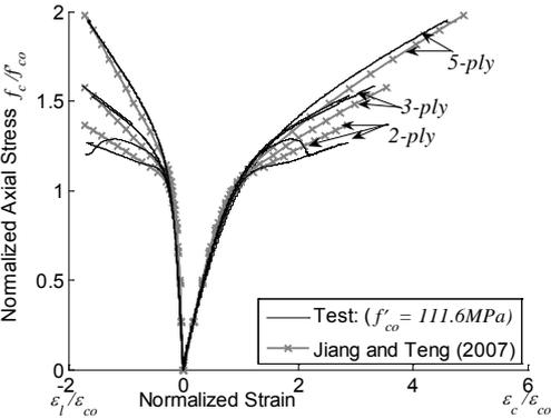
Figure 3 Test and predicted stress-strain curves of CFRP-confined high strength concrete
