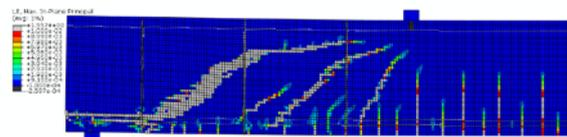
b) Predicted crack pattern at the ultimate state
