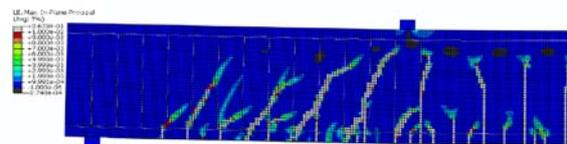
b) Predicted crack pattern at the ultimate state
