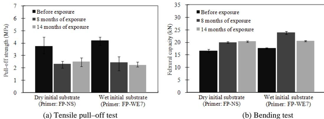
Figure 7 Performance of FRP-to-concrete interfaces after combined wet/dry and thermal cycling
