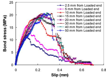
Figure 5 Local bond-slip curves of NSM FRP obtained from finite element analysis
