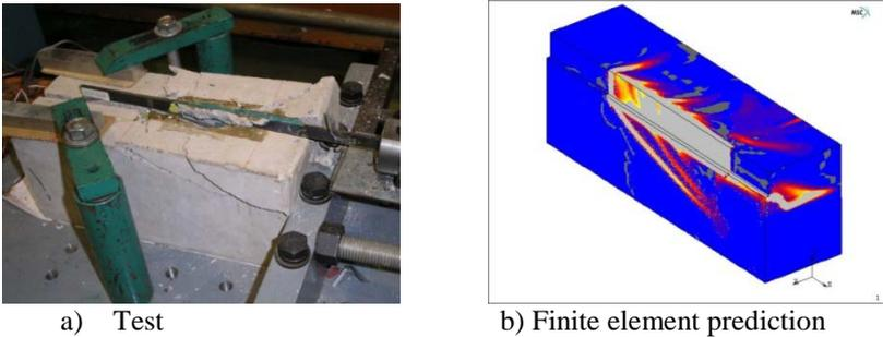
Figure 4 Crack pattern of NSM FRP-to-concrete bonded joint
