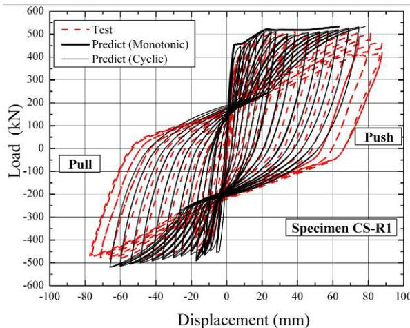
Figure 6 Hysteretic behaviour of an FRP-jacketed RC column
