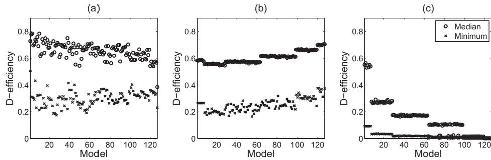
Figure 1: Median and minimum  $D$ -efficiencies for each of the 127 alternative models (ordered from one factor models to the seven factor main effects model) for the (a) compromise  $D$ -optimal design (b)  $D$ -optimal design for the average model and (c) orthogonal design from Wu and Hamada (2000).
