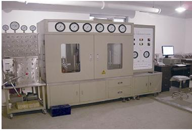
Fig. 1. Constant load creep seepage experiment device.
