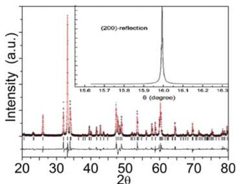
FIG. 1. (Color online) XRD observed (+) and calculated (—) profile, and difference profile (bottom trace) for  $\text{YFeO}_3$  single crystal at room temperature. The bars indicate the diffraction peak positions in the standard. Inset is the profile of the high resolution diffraction peak of the (100) oriented wafer.
