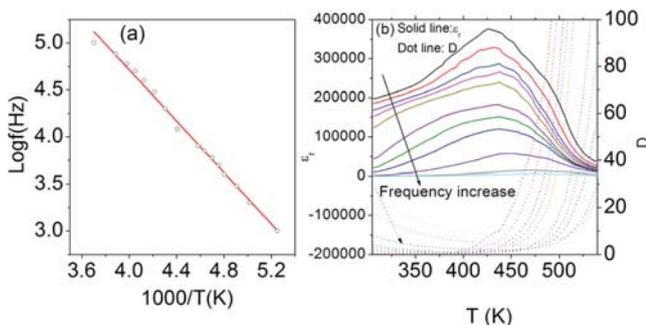
FIG. 5. (Color online) (a) is the Arrhenius plot for the low-temperature relaxation, with the solid line indicating the least squares linear fitting; (b) shows the dielectric behavior in the high temperature range.
