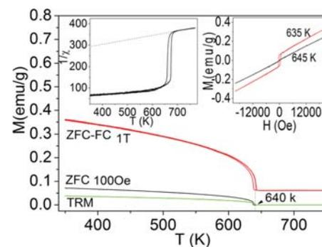
FIG. 3. (Color online) Temperature dependence of the magnetization of  $\text{YFeO}_3$  in fields of 100 Oe and 1 T, and for a thermoremanent magnetization measurement, measured from 310 K to 750 K. Left inset is the Curie-Weiss law fitting for temperatures from 700 to 750 K. Right inset is magnetization vs magnetic field measured at 635 K (below  $T_N$ ) and 645 K (above  $T_N$ ).
