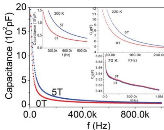
FIG. 6. (Color online) Capacitance of  $\text{YFeO}_3$  single crystal capacitor measured in zero field and 5 T field, at temperatures of 305 (magnified high-frequency part is also shown), 70, and 220 K.
