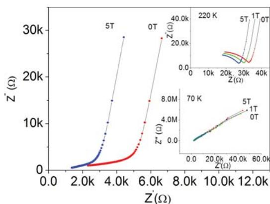
FIG. 7. (Color online) Impedance Cole-Cole plots in zero field and 5 T field of  $\text{YFeO}_3$  single crystal, measured at temperatures of 305, 70, and 220 K. 1 T plots are also shown in the insets.
