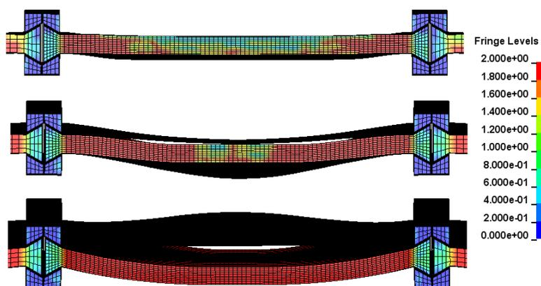
**Figure 6.** The response of the protective barrier with mild steel posts subjected to blast loading due to detonation of 500 kg TNT at 5 m stand-off distance.
