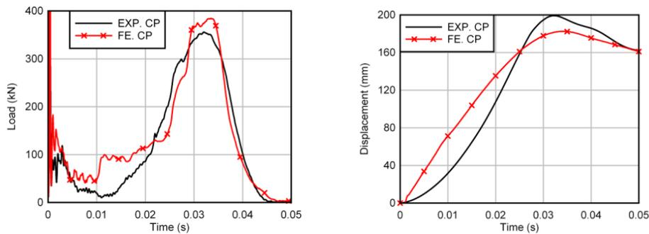
**Figure 3.** A comparison between the experimental and predicted results for the Control panel: (a) impact load time histories, and (b) displacement time histories.
