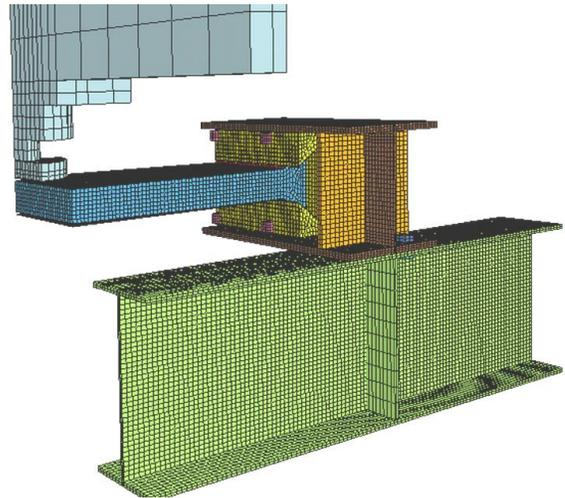
**Figure 2.** LS-DYNA model of experimental setup for SCS sandwich panels
