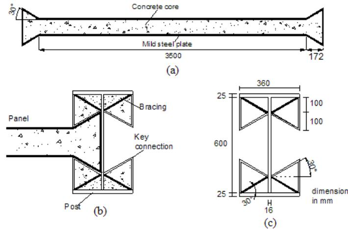
**Figure 1.** Geometry of the prototype barrier system components: (a) sandwich steel-concrete-steel panel with flared ends, (b) keyed connection details, and (c) dimensions of the post.
