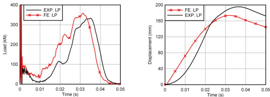
**Figure 4.** A comparison between the experimental and predicted results for the Lightweight core panel: (a) load time histories, and (b) displacement time histories.
