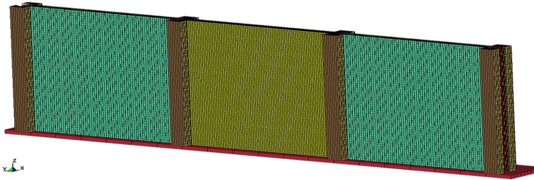
**Figure 5.** FE model of the modular barrier wall system.
