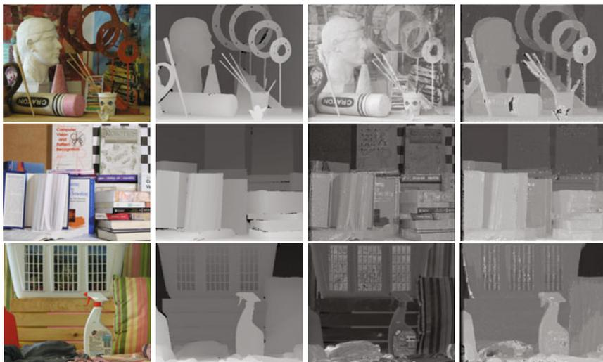
**Fig. 3.** Examples of disparity estimation on Middlebury stereo data sets. Columns from left to right: image, ground-truth,  $SSVR^{cube}$  result scaled for ease of view (original result is pretty dark), and prediction of our approach.
