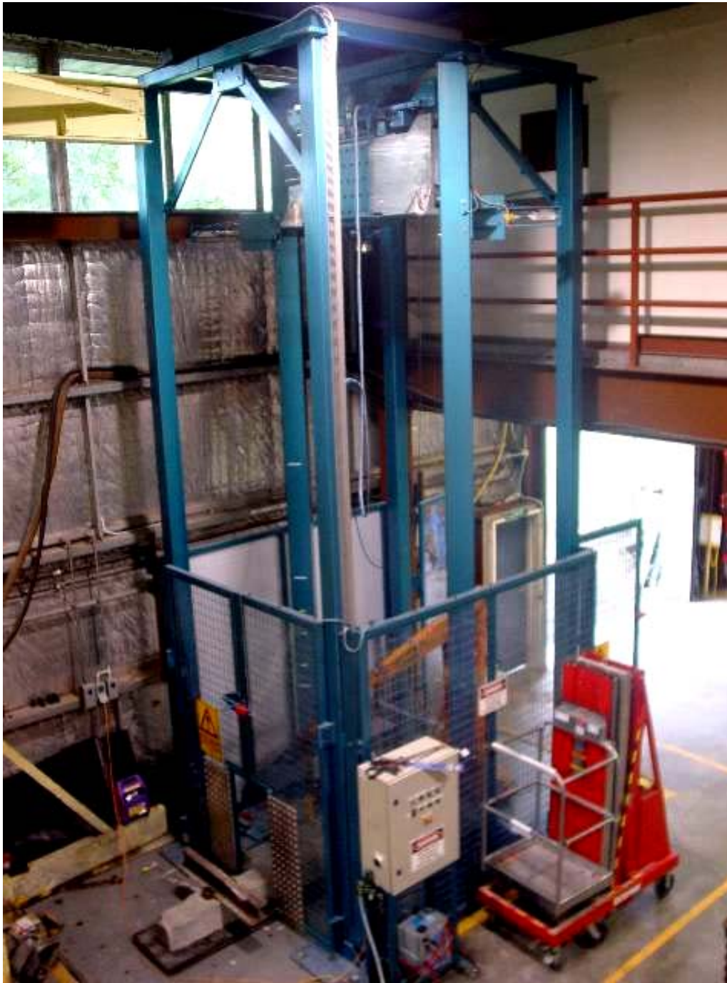
Figure 3 High-capacity drop-weight impact machine at the University of Wollongong
