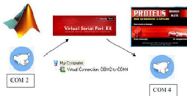
Fig. 10: The virtual interface between Matlab and Proteus
