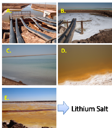
Fig.1. The sequential evaporation pond for the enrichment of lithium at East Taijinar salt-lake brine. The intergranular brine was pumped from underground basin to a trench (A); Brine was further distributed via a reservoir (B); Evaporation by solar power to precipitate sodium chloride (C); the brine after production of potassium chloride, at this stage the lithium concentration was about 2 g/L (D); Further evaporation of the brine enriched the lithium concentration up to 4-5 g/L (E); Finally, The concentrated brine was used for the lithium recovery.
