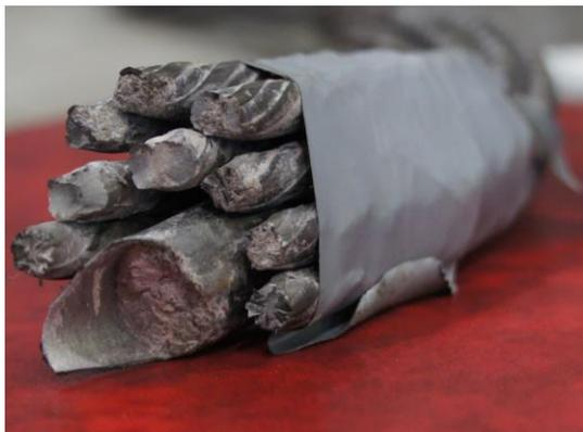
Fig. 7. Tensile and shear failure of cable bolt.
