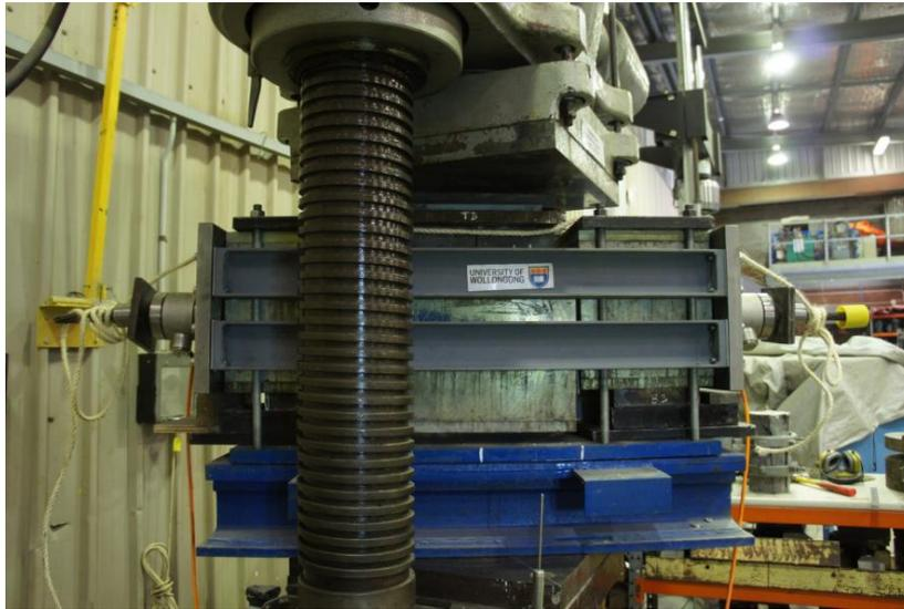
Fig. 2. Double shear assembly without friction between concrete blocks.
