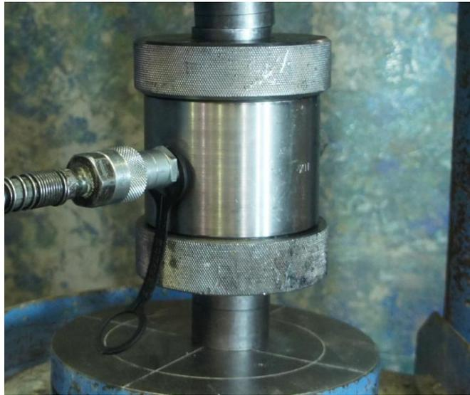
Fig. 6. Triaxial cell in testing arrangement.
