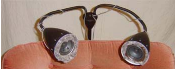
Figure 4. Speaker housed in lampshade with acoustic insulation and gooseneck connection
