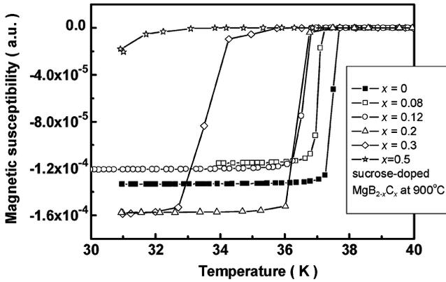
Fig. 1. Magnetic AC susceptibility for  $\text{MgB}_{2-x}\text{C}_x$  as a function of temperature for different carbon doping content. Carbon added was in the form of sucrose ( $\text{C}_{12}\text{H}_{22}\text{O}_{11}$ ). As the doping content increases, the onset transition temperature decreases.
