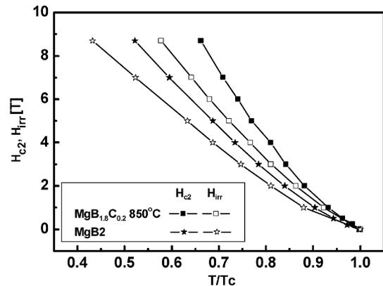
Fig. 7. Normalized temperature ( $T/T_c$ ) dependence of the upper critical field,  $H_{c2}$ , and the irreversibility field,  $H_{irr}$ , for pure  $MgB_2$  and sucrose-doped  $MgB_{1.8}C_{0.2}$ . The latter was sintered at  $850^\circ C$ .
