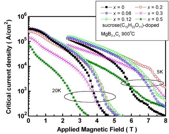
Fig. 2. Critical current density,  $J_c$ , as a function of applied magnetic field for all sucrose-doped samples of  $\text{MgB}_{2-x}\text{C}_x$  at 5 K and 20 K.
