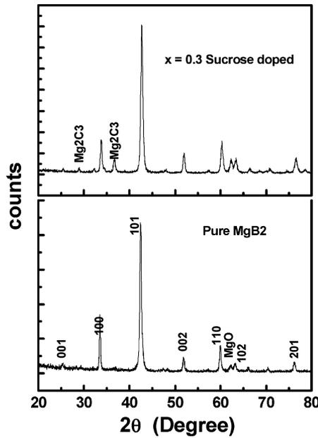
Fig. 4. X-ray diffraction pattern (Cu  $K\alpha$  radiation) for the pure  $MgB_2$  and the sucrose-doped sample  $MgB_{1.7}C_{0.3}$ . The peaks of  $Mg_2C_3$  and  $MgO$  are marked.
