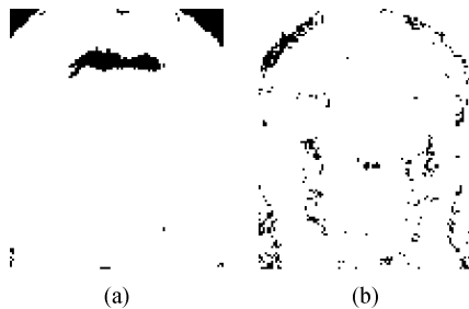
Fig. 5. Pixels selected by (a) NCFS and (b) RCFS (black dots, k = 500 ).
