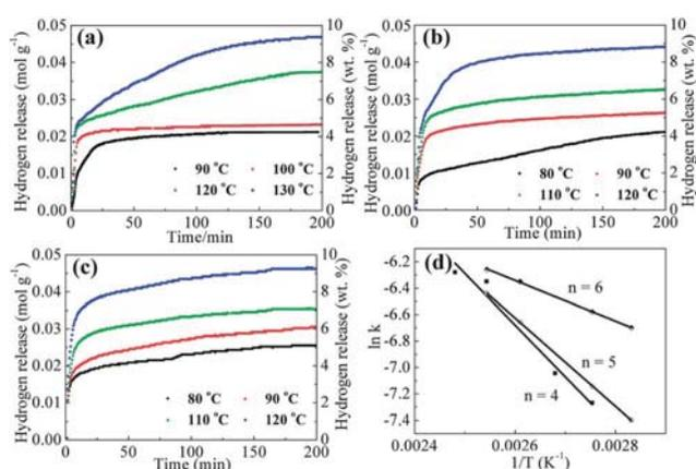
**Fig. 6** Isothermal volumetric measurements of hydrogen release from Li<sub>3</sub>AlH<sub>6</sub>-*n*AB composites when *n* = 4 (a), 5 (b), and 6 (c) at different temperatures, and (d) Arrhenius plots of the temperature-dependent rate data.
