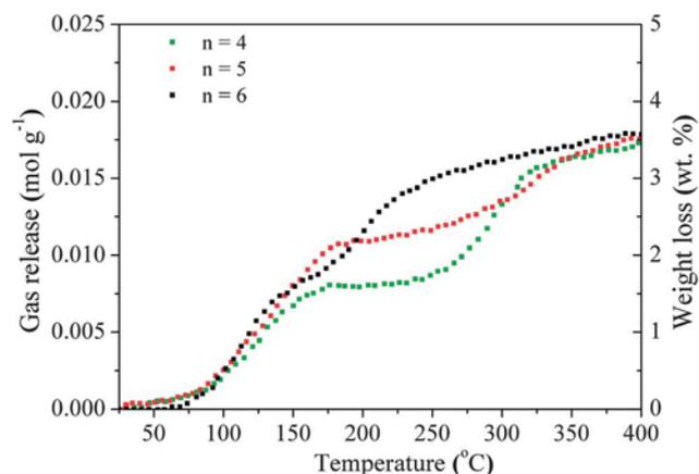
Fig. 13 TPD results for the decomposition of  $\text{Li}_3\text{AlH}_6-n\text{AB}$  ( $n = 4, 5,$  and  $6$ ) composites after regeneration from the spent fuels.
