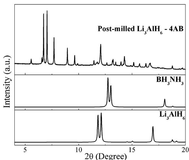
Fig. 1 High-resolution X-ray diffraction pattern of the post-milled Li<sub>3</sub>AlH<sub>6</sub>-4AB composite, with the patterns of pristine AB and Li<sub>3</sub>AlH<sub>6</sub> included for comparison.
