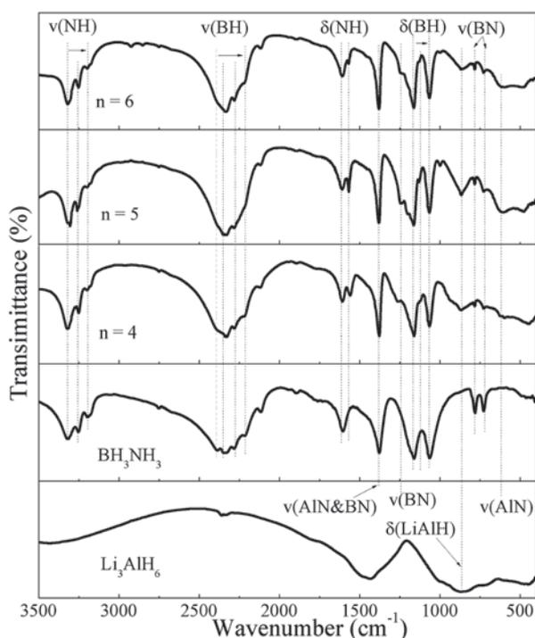
Fig. 3 FTIR spectra of the as-prepared  $\text{Li}_3\text{AlH}_6$ -*n*AB (*n* = 4, 5, and 6) composites, including spectra of pristine AB and as-prepared  $\text{Li}_3\text{AlH}_6$  for comparison.
