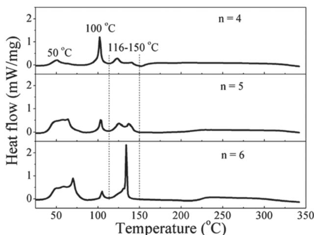
**Fig. 7** Differential scanning calorimetry results for Li<sub>3</sub>AlH<sub>6</sub>-*n*AB (*n* = 4, 5, and 6) composites under a heating rate of 2 °C min<sup>-1</sup> in 1 atm N<sub>2</sub> atmosphere.
