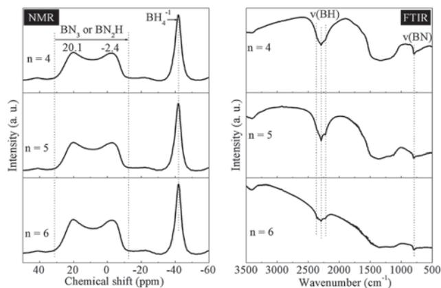
**Fig. 9** Solid-state  $^{11}\text{B}$  NMR and FTIR spectra of  $\text{Li}_3\text{AlH}_6-n\text{AB}$  ( $n = 4, 5,$  and  $6$ ) composites upon heating to  $350\text{ }^\circ\text{C}$  with a heating rate of  $2\text{ }^\circ\text{C min}^{-1}$ .
