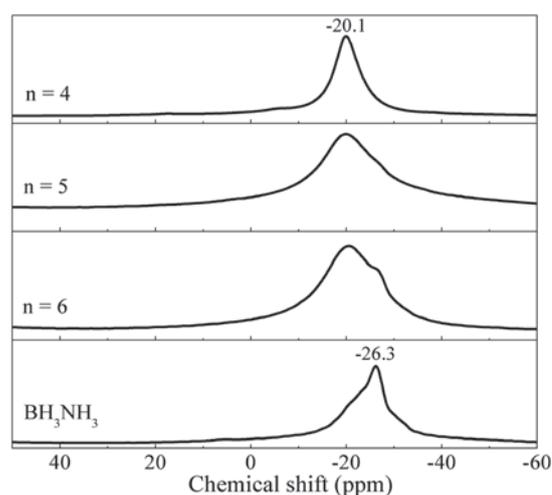
Fig. 2 Solid-state <sup>11</sup>B NMR spectra of the as-prepared Li<sub>3</sub>AlH<sub>6</sub>-*n*AB (*n* = 4, 5, and 6) composites, including pure AB for comparison.
