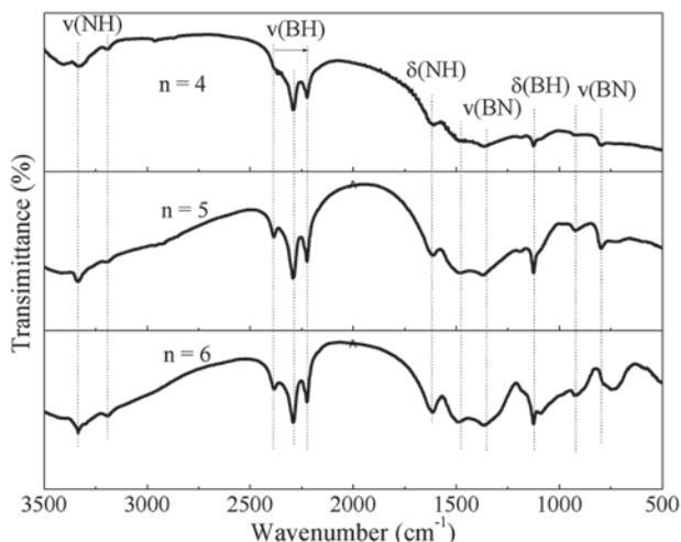
Fig. 11 FTIR spectra of  $\text{Li}_3\text{AlH}_6-n\text{AB}$  ( $n = 4, 5,$  and  $6$ ) composites after regeneration from the spent fuels.
