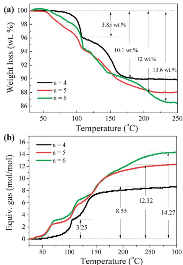
**Fig. 5** (a) TGA and (b) volumetric results for the decomposition of the post-milled  $\text{Li}_3\text{AlH}_6$ - $n\text{AB}$  ( $n = 4, 5,$  and  $6$ ) composites at a heating rate of  $2\text{ °C min}^{-1}$  under 1 atm  $\text{N}_2$  atmosphere.
