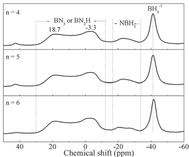
**Fig. 10** Solid-state  $^{11}\text{B}$  NMR spectra of  $\text{Li}_3\text{AlH}_6-n\text{AB}$  ( $n = 4, 5,$  and  $6$ ) composites after regeneration from the spent fuels.
