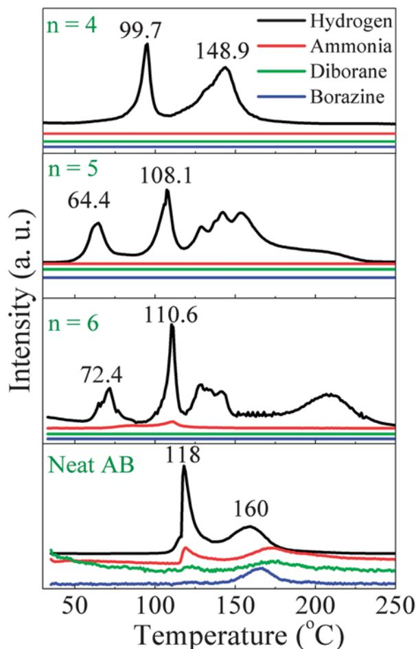
**Fig. 4** MS spectra of the as-prepared  $\text{Li}_3\text{AlH}_6$ - $n\text{AB}$  ( $n = 4, 5,$  and  $6$ ) composites with a heating rate of  $2\text{ °C min}^{-1}$  under 1 atm dynamic  $\text{N}_2$  atmosphere, including neat AB for comparison.
