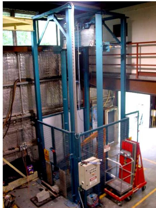
Fig.4 Impact testing facility
