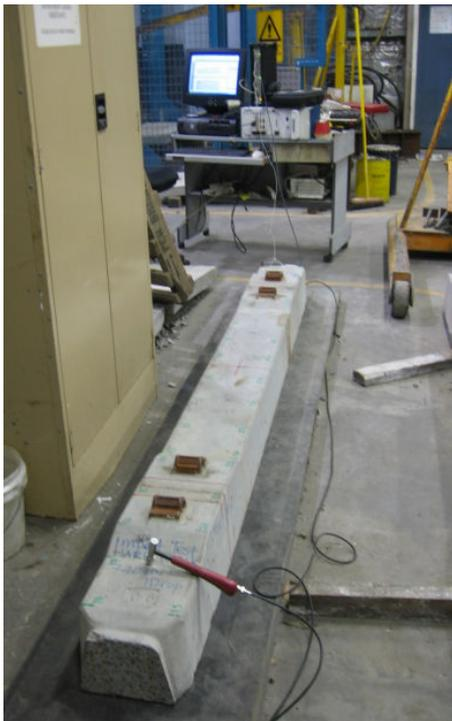
Fig. 3 Modal testing setup
