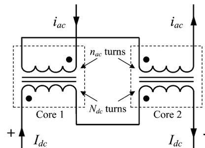
Fig. 1. Basic configuration of a saturable core-type FCL.
