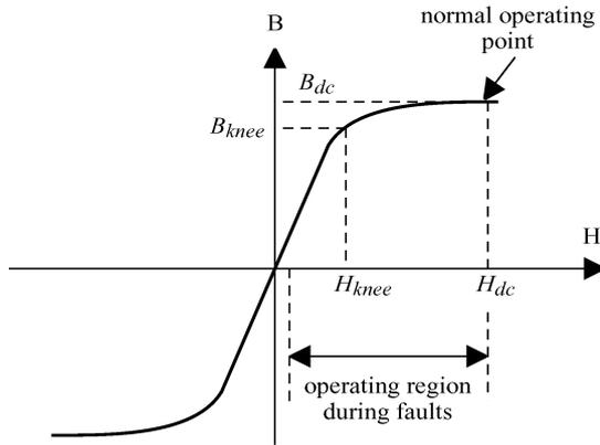
Fig. 2. Operating region of the saturable core-type FCL.
