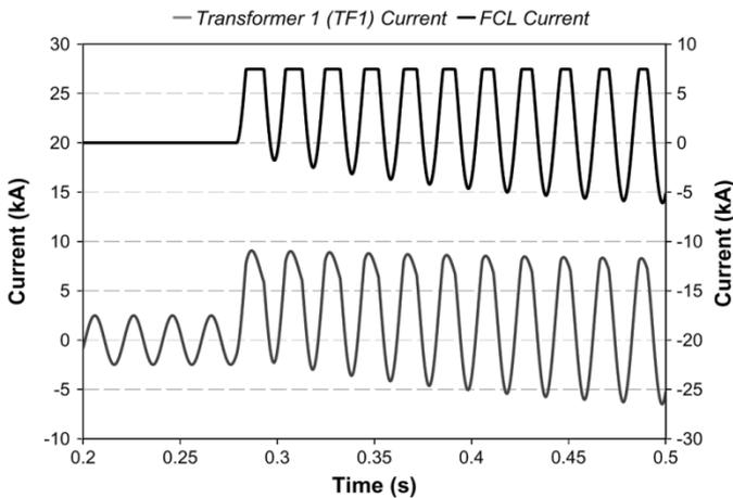
Fig. 12. Substation arrangement 2 transformer currents during fault ( $N_{dc} = 560$  turns,  $I_{dc} = 400$  A,  $n_{ac} = 30$  turns).
