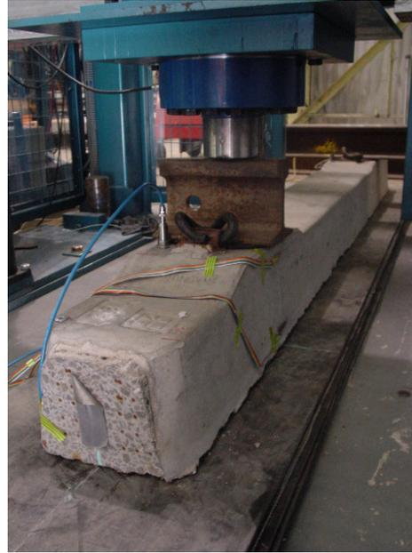
b) impact test setup
