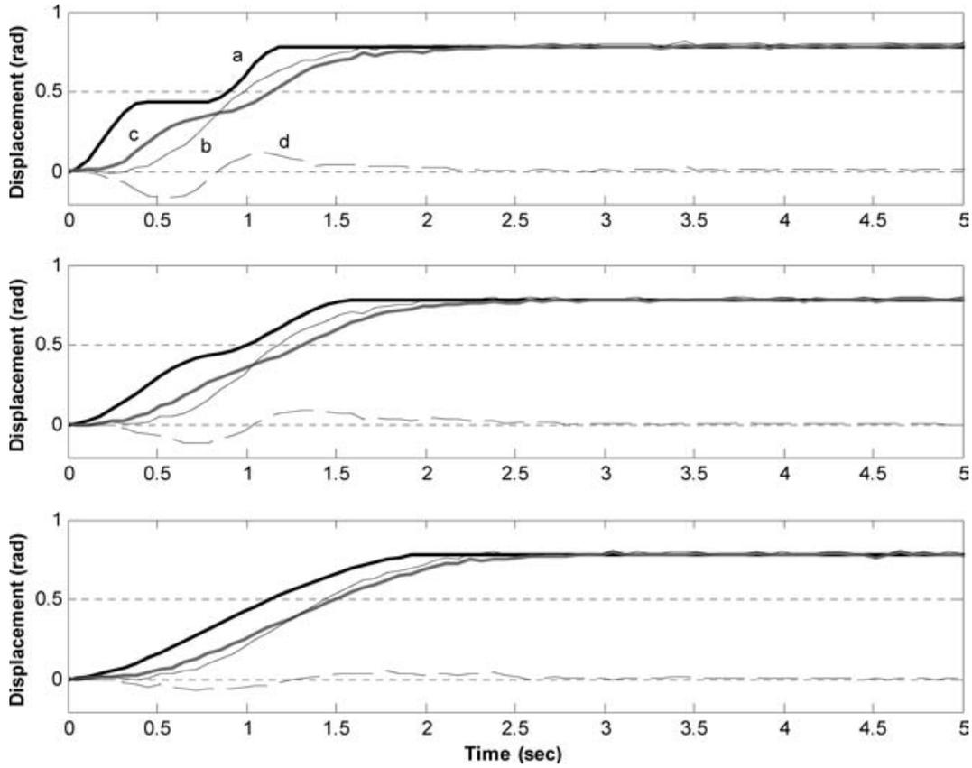
Fig. 8. Experimental results from the hybrid input shaping technique for a traveling distance of  $\theta = \pi/4$  rad.  $\theta_1$  and  $\theta_2$  are arbitrarily taken as  $\pi/8$  and  $\pi/8$  radians, respectively, and for the traveling times of (a),  $\tau_t = 1.5\pi/\omega_n$  seconds, (b)  $\tau_t = 2.0\pi/\omega_n$  seconds, and (c)  $\tau_t = 2.5\pi/\omega_n$  seconds.
