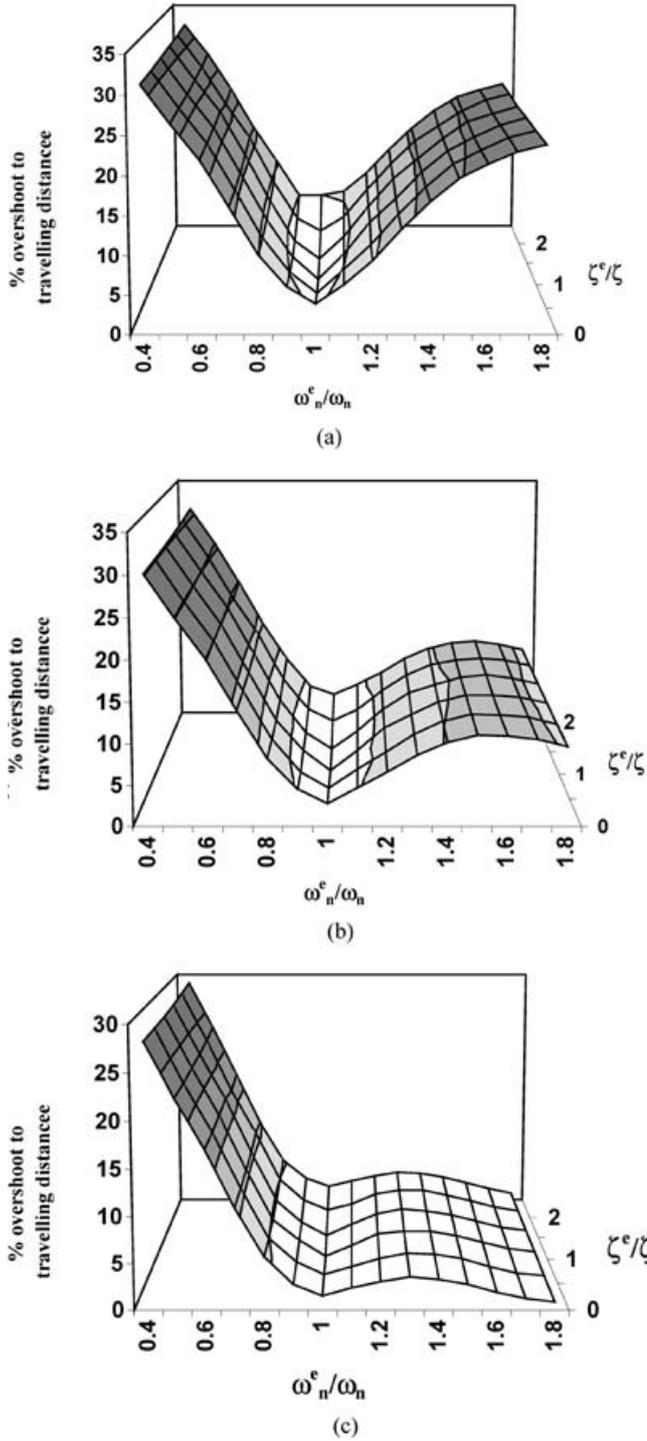
Fig. 4. Simulated sensitivity of the system to uncertainties in the system natural frequency and damping ratio for a total traveling distance of  $\theta = \pi/4$  rad.  $\theta_1$  and  $\theta_2$  are arbitrarily taken as  $\pi/8$  and  $\pi/8$  radians, respectively. The plot (a) is for  $\tau_t = 1.5\pi/\omega_n$  seconds, the plot (b) is for  $\tau_t = 2.0\pi/\omega_n$  seconds, and the plot (c) is for  $\tau_t = 2.5\pi/\omega_n$  seconds.
