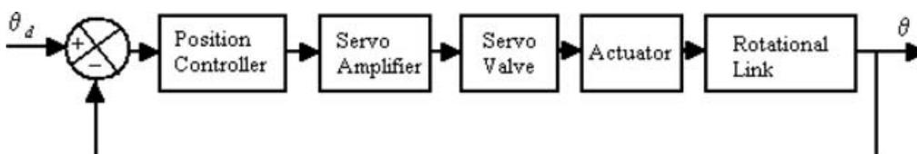
Fig. 7. Control strategy for the position control of the rotational link of the manipulator shown in Figure 6.
