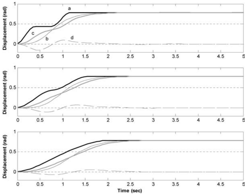
Fig. 2. Simulation results from the hybrid input shaping technique for a traveling distance of  $\theta = \pi/4$  rad.  $\theta_1$  and  $\theta_2$  are arbitrarily taken as  $\pi/8$  and  $\pi/8$  radians, respectively, and for the traveling times of  $\tau_t = 1.5\pi/\omega_n$  seconds (top plot),  $\tau_t = 2.0\pi/\omega_n$  seconds (middle plot), and  $\tau_t = 2.5\pi/\omega_n$  seconds (bottom plot).
