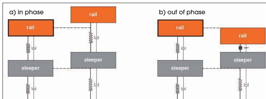
Figure 2: Simplification of railway track dynamics: a) in phase; b) out of phase.
