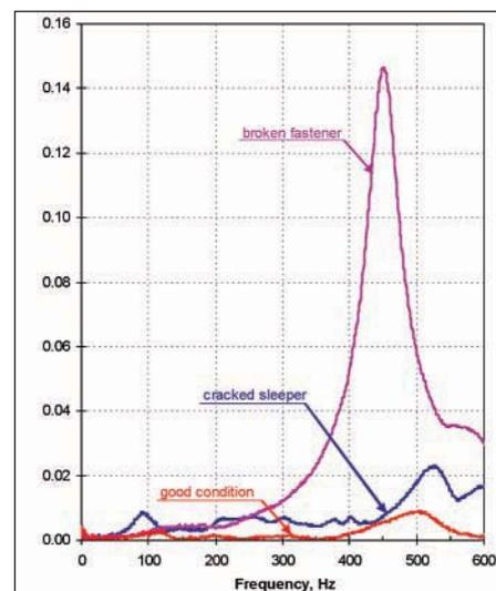
Figure 6: Frequency response function (FRF) of railway track structures.
