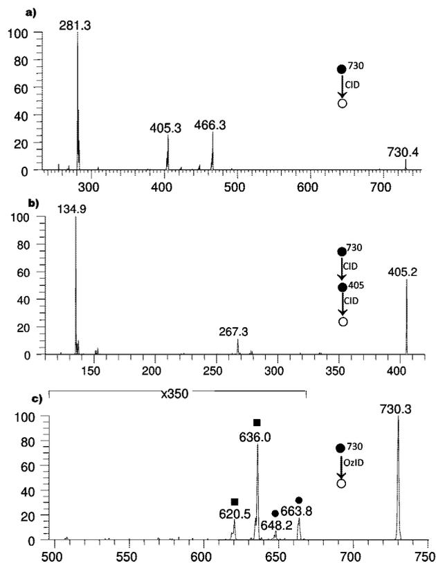
**Figure 4.** Negative ion electrospray ionization mass spectra obtained using a linear quadrupole ion-trap mass spectrometer: (a) CID of the GPEtn at  $m/z$  730, (b) CID of the  $m/z$  405 fragment ion produced in (a) (i.e.,  $730 \rightarrow 405 \rightarrow \text{CID}$ ), and (c) OzID of  $m/z$  730. ■ = OzID ions produced from oxidative cleavage of  $n$ -9 double bonds. ● = OzID ions produced from oxidative cleavage of  $n$ -7 double bonds.
