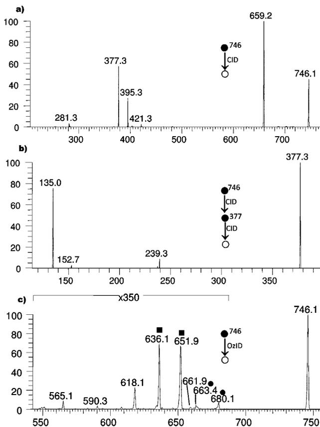
**Figure 5.** Negative ion electrospray ionization mass spectra obtained using a linear quadrupole ion-trap mass spectrometer: (a) CID of the GPSer at  $m/z$  746, (b) CID of the  $m/z$  377 fragment ion produced in (a) (i.e.,  $746 \rightarrow 377 \rightarrow \text{CID}$ ), and (c) OzID of  $m/z$  746. ■ = OzID ions produced from oxidative cleavage of  $n$ -9 double bonds. ● = OzID ions produced from oxidative cleavage of  $n$ -7 double bonds.
