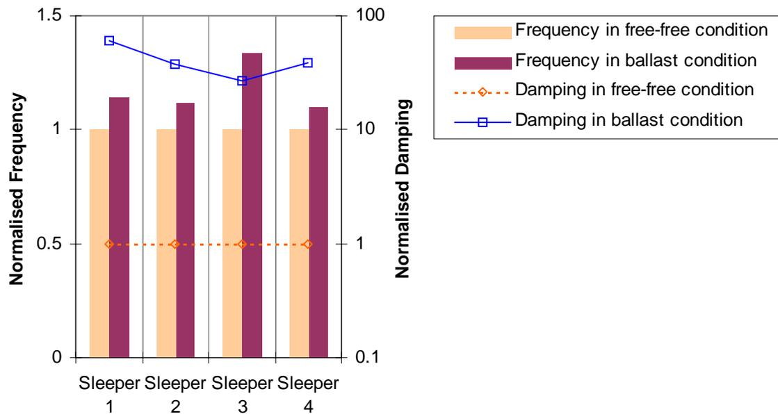
Figure 5 Effect of boundary conditions on fundamental vibration properties of sleepers
