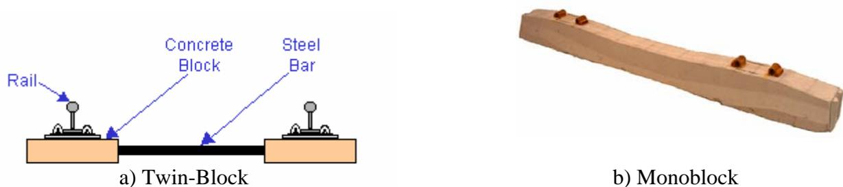
**Figure 2** Concrete sleepers
