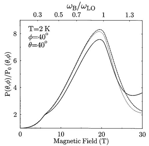
FIG. 6. Dependence of LO-phonon emission on parallel magnetic field for different electron temperatures:  $T_e = 40$  (solid curve), 50 (dotted curve), and 60 K (dashed curve).  $P_0(\theta, \phi)$  is the phonon intensity at  $B=0$ . The sample parameters are the same as in Fig. 1.
