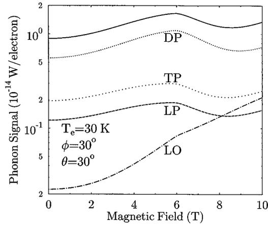
FIG. 2. Total intensity of phonon signal (solid curve) and the contribution from different phonon modes as a function of parallel magnetic field at electron (lattice) temperature  $T_e = 30$  K ( $T = 2$  K). The sample parameters are the same as Fig. 1.
