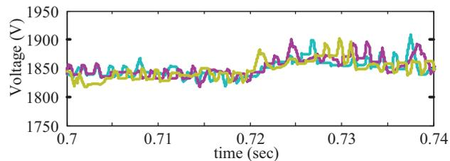
Fig. 10. Variation of cell two capacitor during a step change in active power
