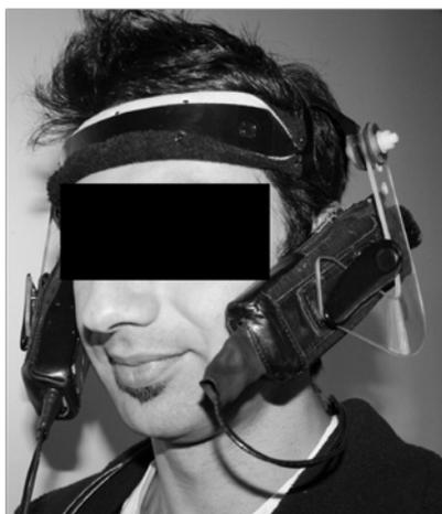
Fig. 3. The head cradle supports two mobile phone devices with the one next to the right side of the head radiating while the one on the left was inactive. The devices were otherwise identical in appearance and weight.
