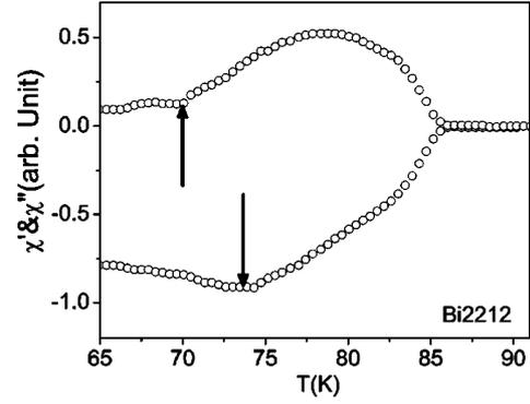
FIG. 8. The experimental ACS curves for Bi2212. It is clear that two dips marked by arrows occur at different temperatures and a large broad peak appears in  $\chi''(T)$  curve, conforming the numerical results (see Fig. 3).  $f = 500$  Hz,  $B_{dc} = 170$  Gs and  $B_{ac} = 5$  Gs.
