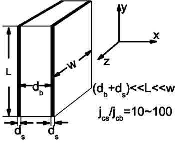
FIG. 1. Schematic sketch for our model. The surfaces are blacked and have critical current density  $j_{cs}$ , while the bulk zone has weak pinning with  $j_{cb}$ . The strength of surface barrier is adjusted by  $j_{cs}/j_{cb}$ , and the width of surface is adjusted by  $d_s/d_b$ .
