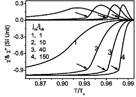
FIG. 2. Numerical ACS curves at different strengths of surface barrier (different  $j_{cs}/j_{cb}$ ) for the critical state model. The kinks indicated by arrows reflect the influence of surface barrier on ACS without flux creep.  $f = 100 \text{ Hz}$ ,  $B_{dc} = 1000 \text{ Gs}$ ,  $B_{ac} = 10 \text{ Gs}$ ,  $d_s/d_b = 0.1$ .
