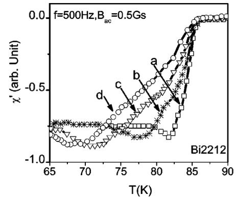
FIG. 9. The real part of experimental ACS curves for Bi2212 at different dc fields. The dip width increases with dc field while its depth is almost unchanged, consistent with the numerical results (see Fig. 4).  $B_{dc}$ : a=50 Gs, b=90 Gs, c=200 Gs, d=300 Gs.
