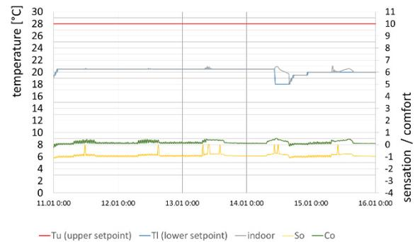
Figure 5. Adjusting the lower set point temperature
