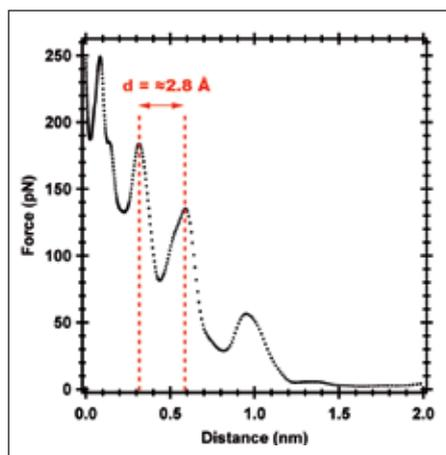
Fig. 3. FM-AFM force curve taken on gel phase DPPC bilayer in pure water at 24 °C.
