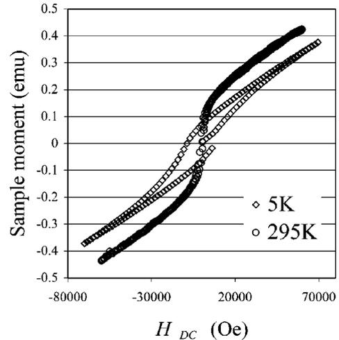
FIG. 1.  $M$ - $H$  loops for a polycrystalline sample of  $Y_{0.33}Sr_{0.67}CoO_{2.79}$  at 5 and 295 K.
