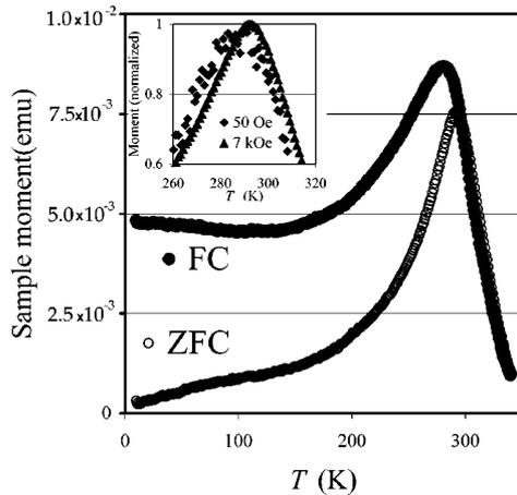
FIG. 2. Zero-field cooled (ZFC) and field cooled (FC) magnetizations against  $T$  for a polycrystalline sample  $Y_{0.33}Sr_{0.67}CoO_{2.79}$  in a field of 7 kOe. Inset shows ZFC measurements in fields of 50 Oe and 7 kOe normalized to demonstrate the constant cusp width.
