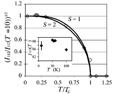
FIG. 6. (Magnetic intensity)<sup>(1/2)</sup> vs reduced temperature plotted for the (112) magnetic Bragg peak. Brillouin curves for  $S=1$  and  $S=2$  are included. Marker size in main figures gives error bars; an indicative error bar is shown in the inset.
