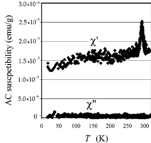
FIG. 3. ac susceptibility of a polycrystalline sample of  $Y_{0.33}Sr_{0.67}CoO_{2.79}$  with  $H_{AC} = 6.25$  Oe,  $H_{DC} = 0$ , and  $f = 125$  Hz.
