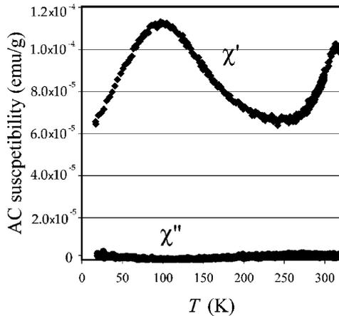
FIG. 4. ac susceptibility of  $Y_{0.1}Sr_{0.9}CoO_{3-\delta}$ , demonstrating the same features as Fig. 3 but the larger feature at 100 K, possibly larger due to the larger fraction of  $Co^{4+}$  ( $\sim 45\%$ ).
