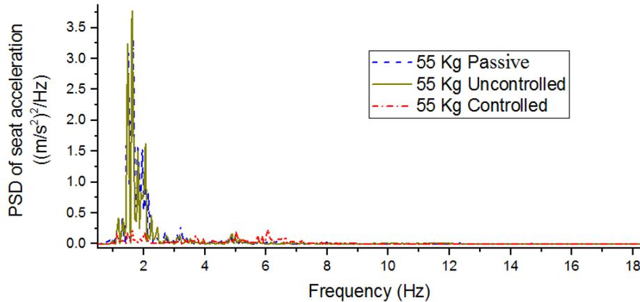
Fig. 15. PSD of vibration with 55 Kg load
