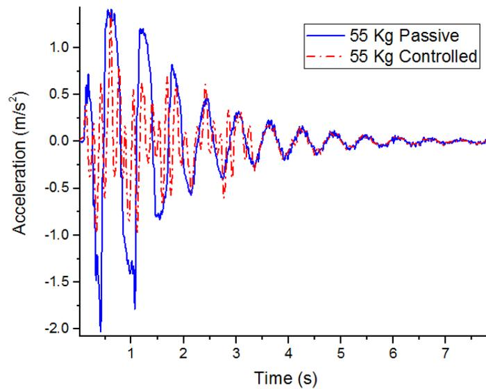
Fig. 11. Bump excitation with 55 Kg load.
