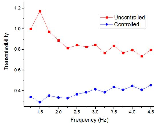
Fig. 8. Simulation acceleration transmissibility of seat suspension
