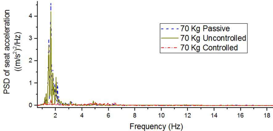
Fig. 16. PSD of vibration with 70 Kg load
