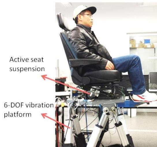
Fig. 9. Experimental setup
