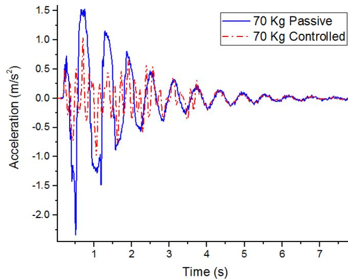
Fig. 12. Bump excitation with 70 Kg load
