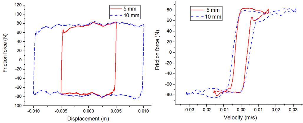
Fig. 18. Displacement-force and velocity-force plot of friction
