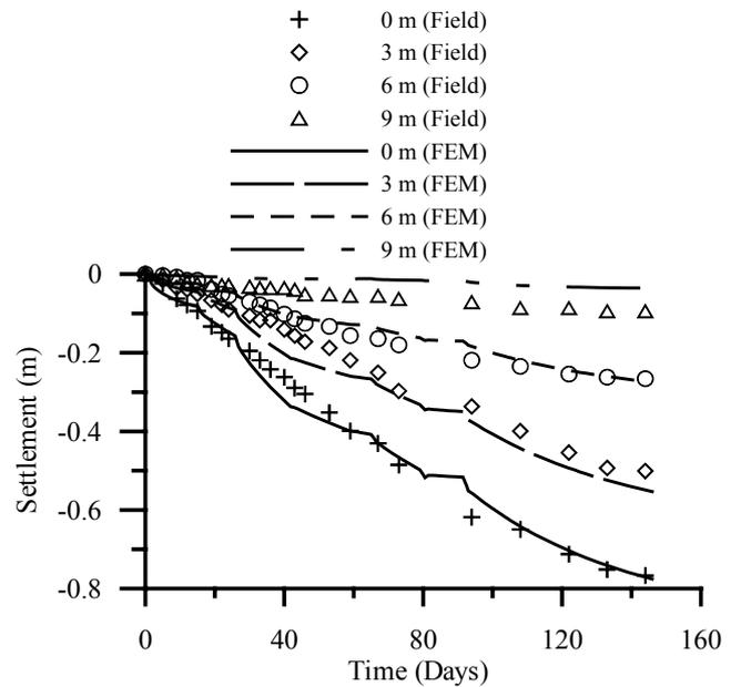
Fig. 12. Consolidation settlement of embankment TV1 (Case C)
