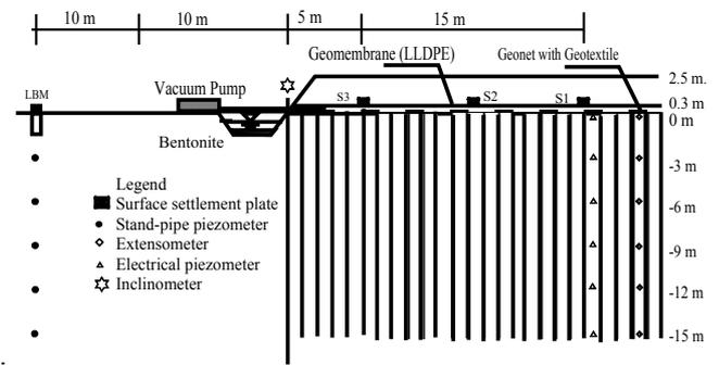
Fig. 5. Cross section of embankment TV1 and location of monitoring system
