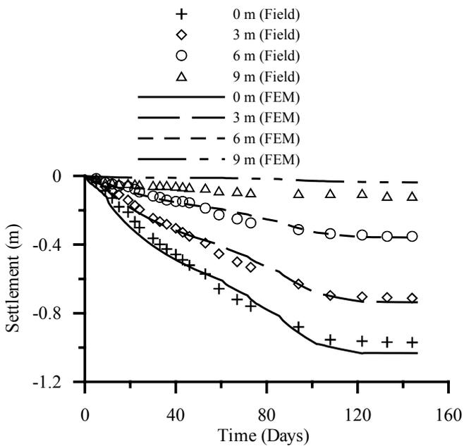
Fig. 14. Consolidation settlement of embankment TV2 (Case C)
