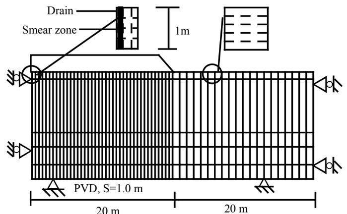
Fig. 8. Finite element mesh for plane strain analysis
