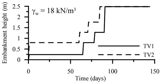
Fig. 7. Multistage loading for embankments TV1 and TV2
