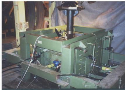
Figure 17. Large-scale prismatic triaxial equipment built at the University of Wollongong
