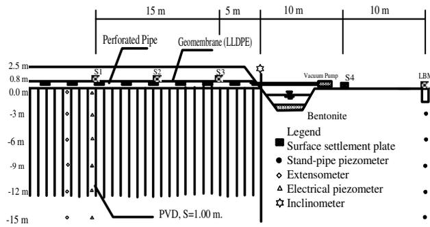
Figure 12: Cross section of embankment TV2 and location of monitoring system (Indraratna et al., 2005d)
