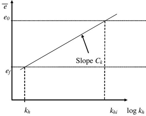
Figure 3: Semi-log permeability-void ratio (after Indraratna et al., 2005b)
