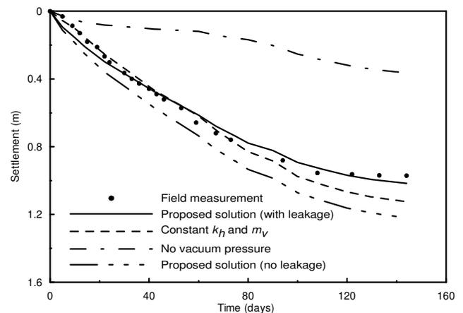
Figure 17: Surface settlement predictions at the centerline of Embankment TV2 (after Rujikiatkamjorn, 2005)
