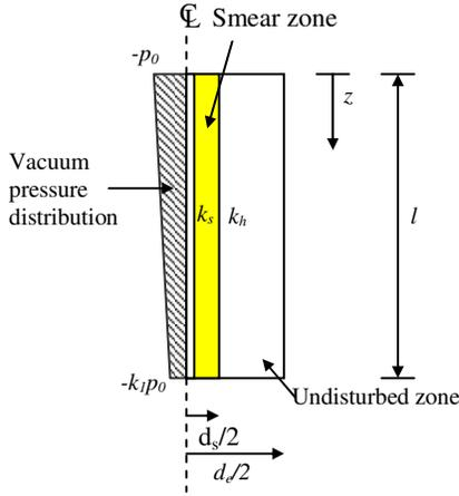
Figure 4: An axisymmetric unit cell with vacuum pressure distribution (modified after Indraratna et al., 2005c)
