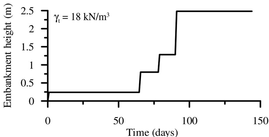
**Figure 10. Multistage loading for embankment TV1 (modified after Indraratna *et al.*, 2005b).**
