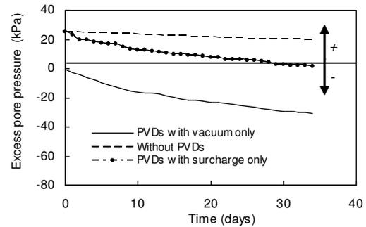
**Figure 8. Time-dependent excess pore water pressure dissipation**
