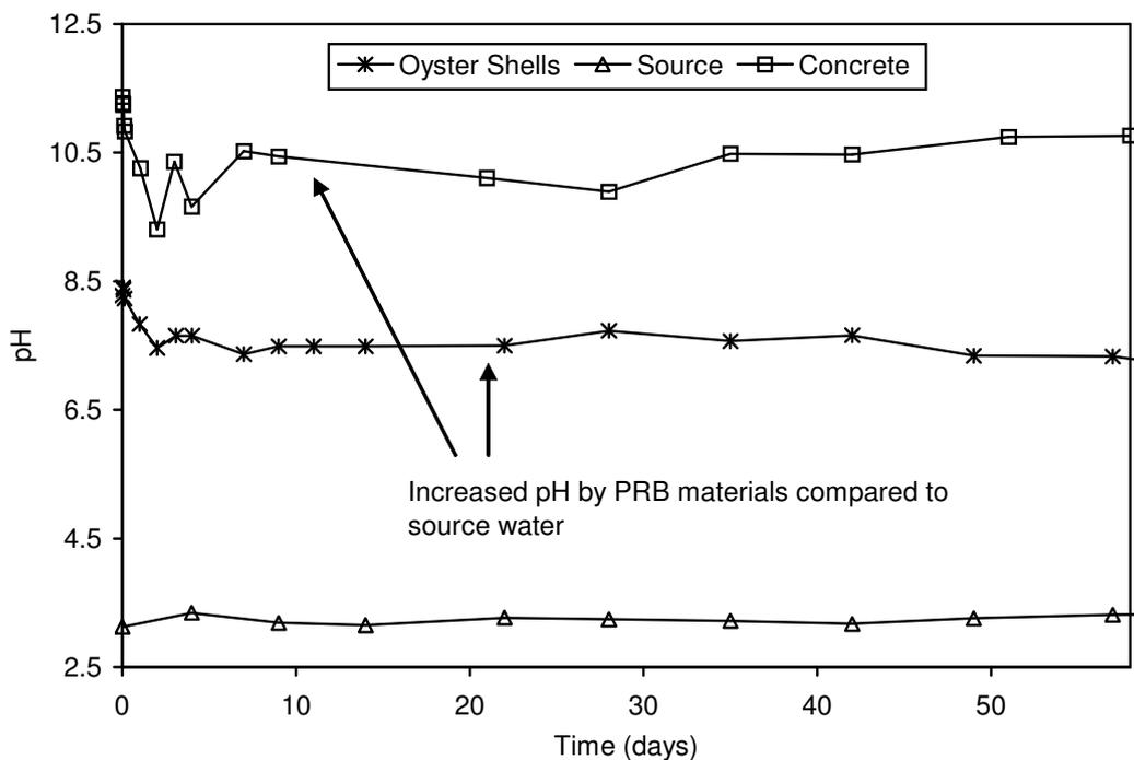
**Figure 3: Performance of oyster shells and recycled concrete in column tests with acidic water over a period of 58 days.** (The source water flowing into the columns and the effluent flowing out of the columns are displayed. Note the neutralising ability of both materials).
