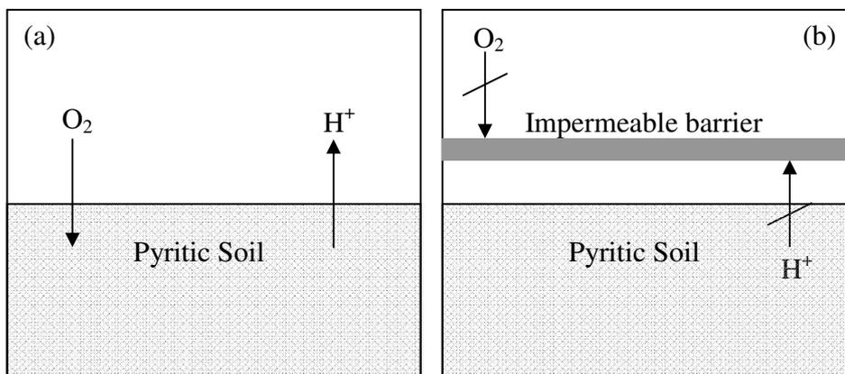
**Figure 2: Schematic of (a) pyritic soil being oxidised by oxygen and releasing acidity into the groundwater and (b) an impermeable horizontal alkaline barrier that prevents the infiltration of oxygen into the pyritic soil and neutralises acidity in the groundwater.**
