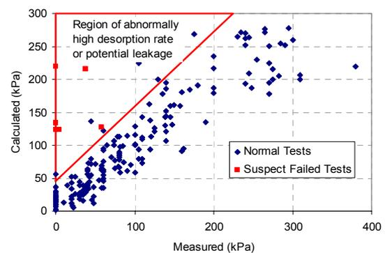
**Fig. 6 Identifying Abnormal Data Based on Canister Pressure**
