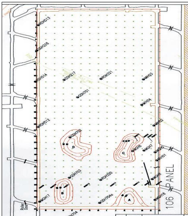
FIG 6 - Underground heating zones identified with radon technique.
