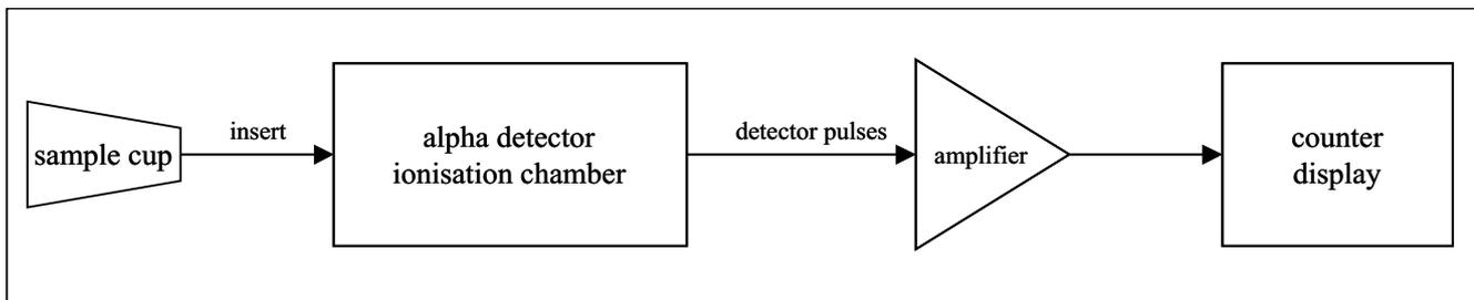
FIG 2 - Working principle of 'alpha cup' method.
