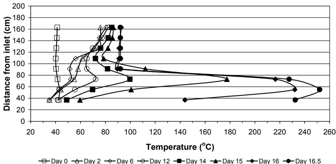
FIG. 4 - Temperature profile of a high-volatile bituminous coal self-heating in the UQ 2-metre column
