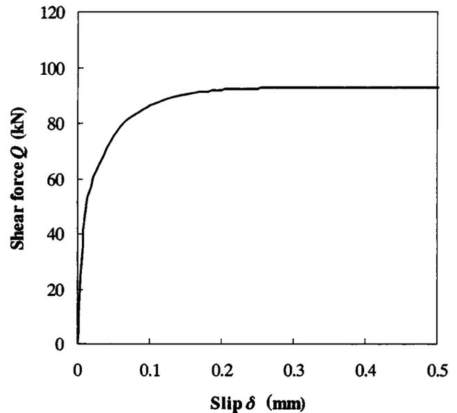
Fig. 3. Shear–slip curve for stud shear connectors
