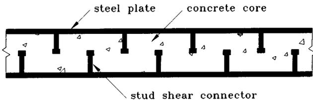
Fig. 1. Cross section of double skin composite panel
