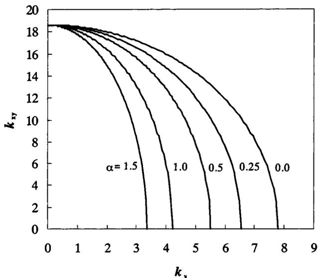
Fig. 7. Buckling interaction curves of plates (C-C-S-S+SC),  $a/b = 1$
