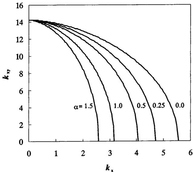
Fig. 6. Buckling interaction curves of plates (C-S-S-S+SC),  $a/b = 1$
