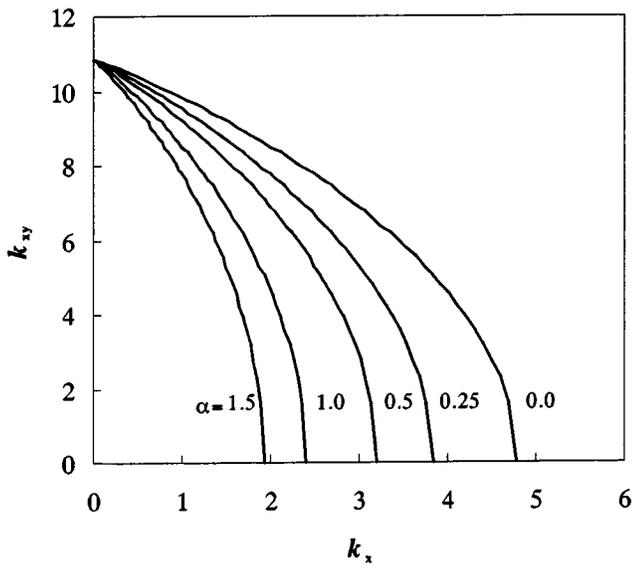
Fig. 4. Buckling interaction curves of plates (S-S-S-S+SC),  $a/b = 1$
