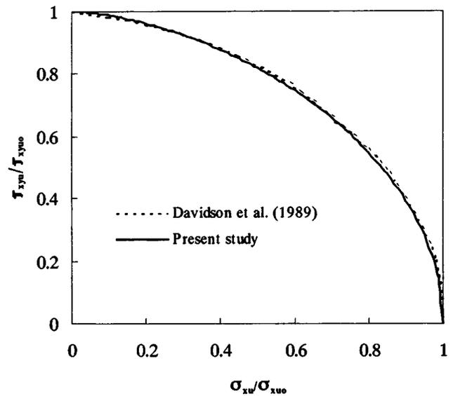
Fig. 11. Comparison of present study with existing results for plate with  $b/t=40$ ,  $a/b=1$ ,  $\alpha=1$
