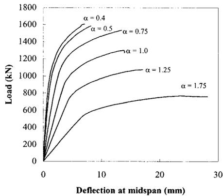
Fig. 7. Load–deflection curves of composite beams with various moment/shear ratios
