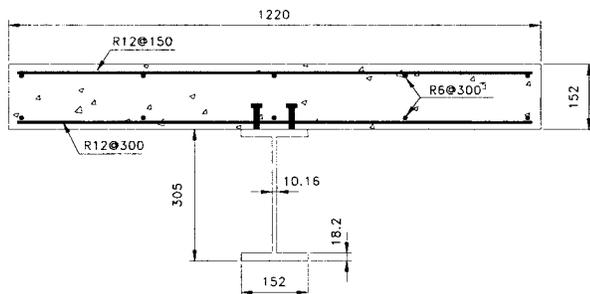
Fig. 5. Cross section of the composite beam
