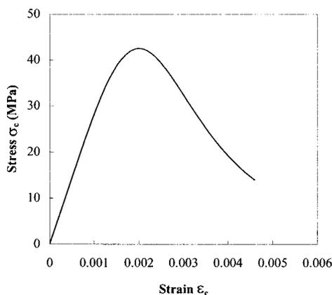
Fig. 3. Stress-strain curve for concrete in compression
