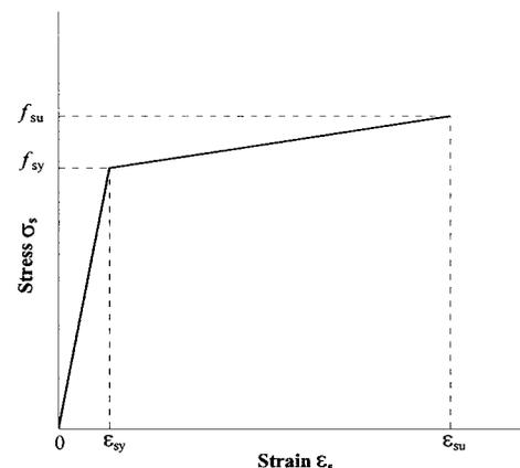
Fig. 2. Stress–strain curve for steel with strain hardening
