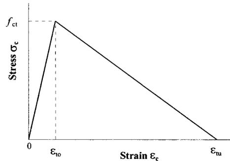
Fig. 4. Stress-strain curve for concrete in tension
