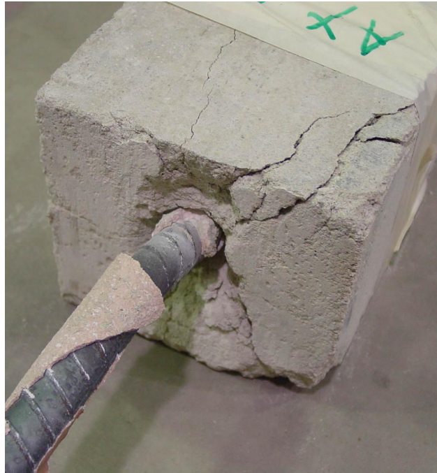
FIG. 6 - Post test end block view of bolt pulled through the concrete during shear loading
