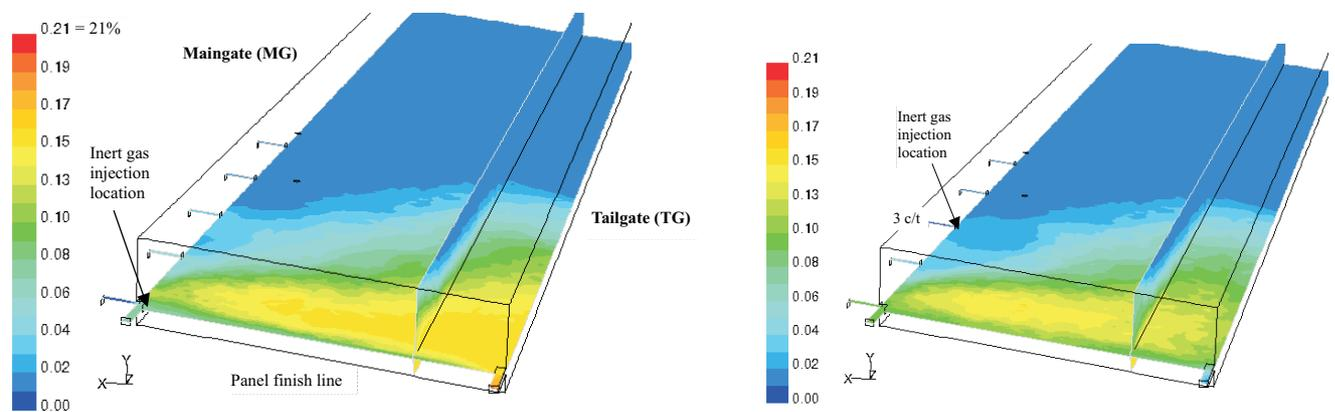
FIG 6 - Oxygen distribution in the goaf – with inert gas through MG seal and 3 c/t seal respectively.
