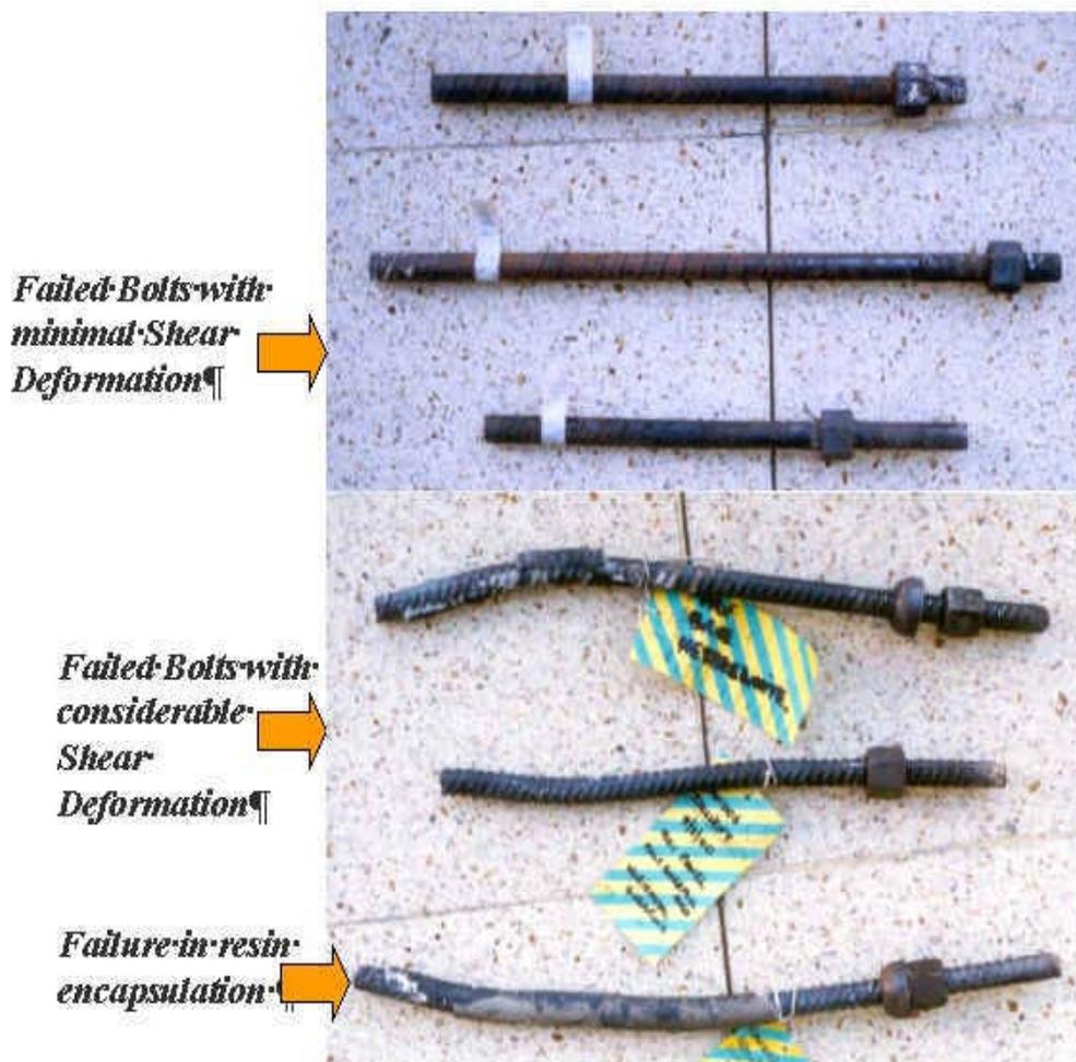
FIG. 2 - SCC Brittle Failures of Rock Bolts
