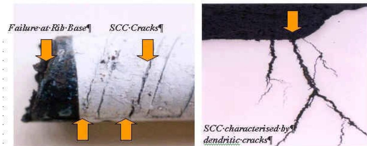
FIG. 1 - SCC Cracking in a Rock Bolt
