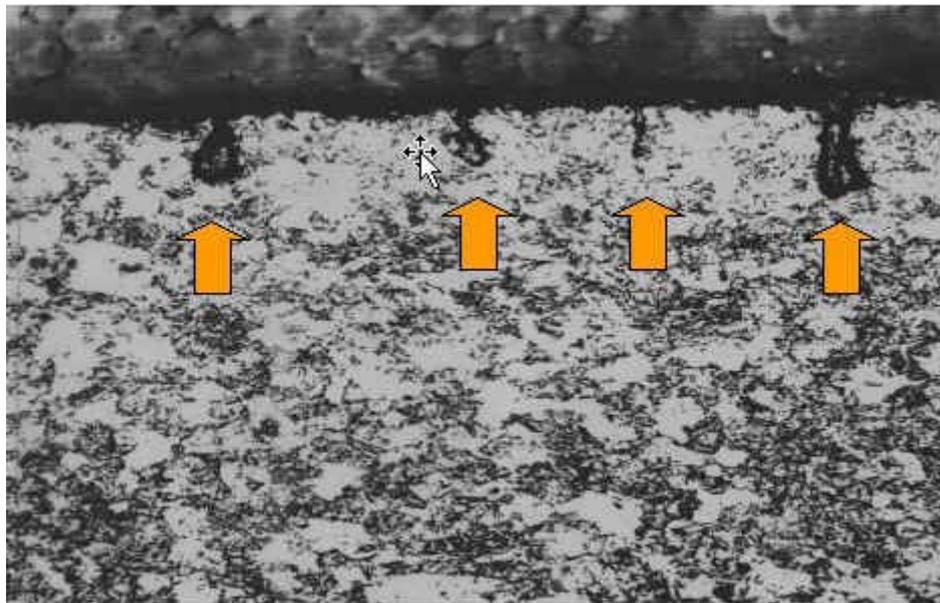
**FIG. 3 - Corrosion Pitting on the bolt surface – may also be an incipient failure point for rock bolts.
