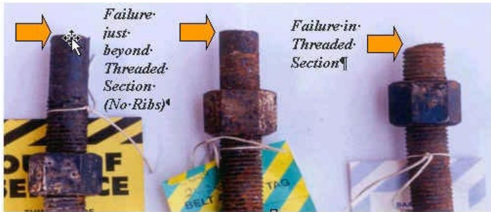
**FIG. 4 - SCC Brittle failures of Rock Bolts near the collar** – the two bolts on the left have failed through the bar-peeled or swaged section of the bolt, whereas the bolt on the right has failed through the root diameter of the thread.
