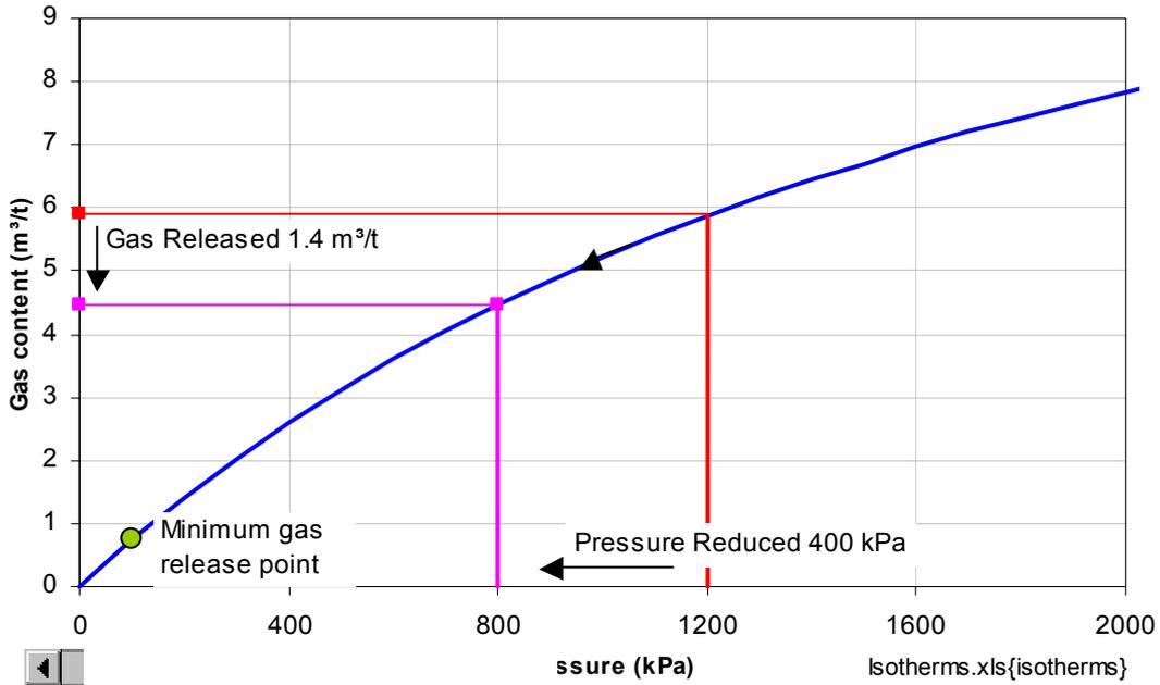
FIG. 5 – Sorption Isotherm Indicating Gas Release with Pressure Reduction
