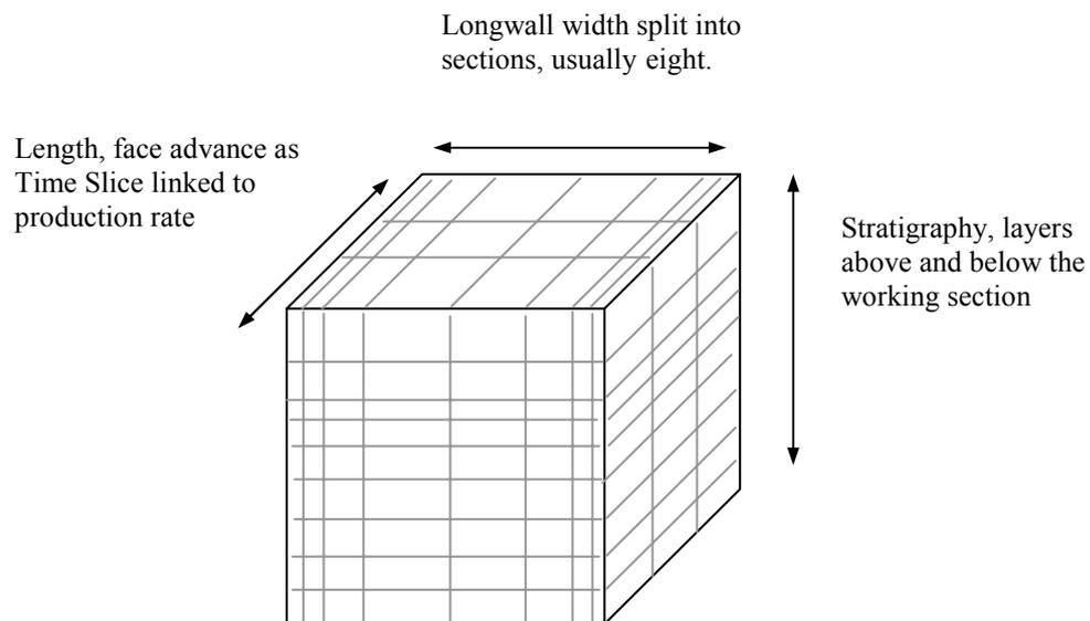
**FIG. 1 – Simplified Block Arrangement for Longwall Model**
