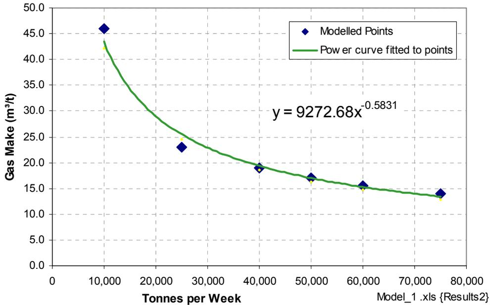
FIG. 7 – Gas Make Curve Plotted from Model Results
