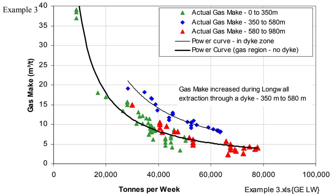
FIG. 8 - Gas Make Curves of Actual Longwall's
