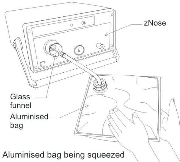
FIG 2 - Sampling from an aluminised bag.
