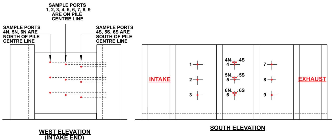
FIG 6 - Coal pile sample tube location and identification.
