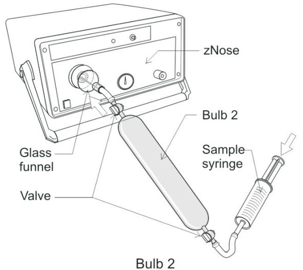
FIG 3 - Sampling from a glass gas bulb.
