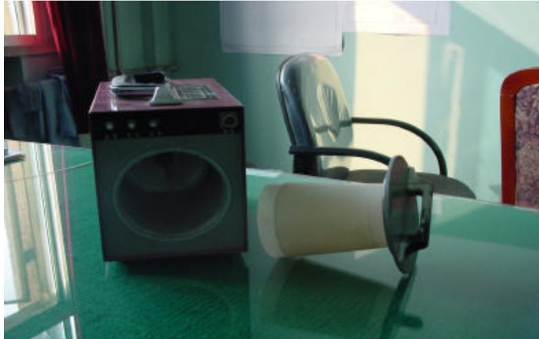
Fig 1 - Alpha cup and CD-1 radon detector
