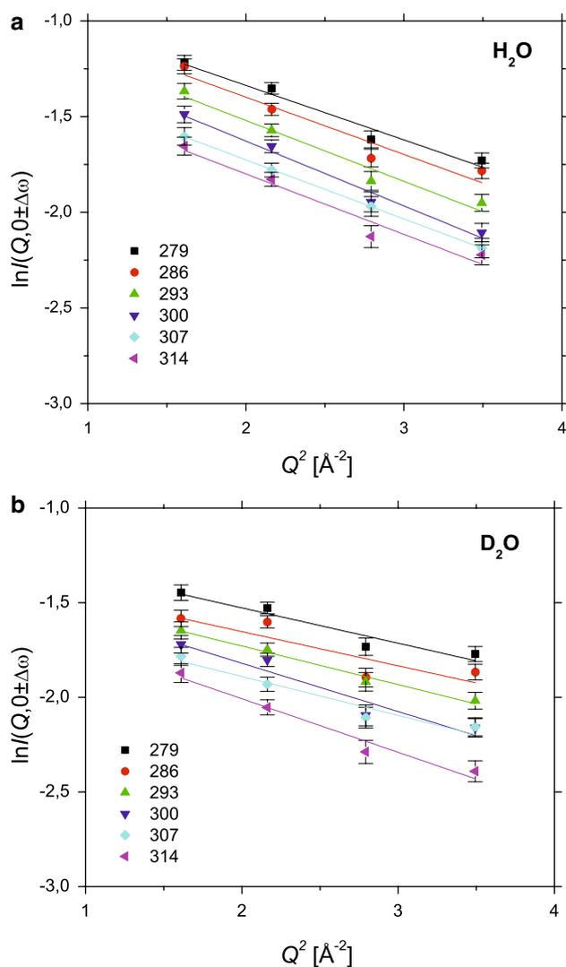
**Fig. 1** Scattered normalized intensities plotted as  $\ln I(Q, \theta \pm \Delta\omega)$  as a function of  $Q^2$  from cells in  $\text{H}_2\text{O}$  (a) and  $\text{D}_2\text{O}$  (b). Linear fits were performed over the ranges  $1.6 \text{ \AA}^{-2} < Q^2 < 3.5 \text{ \AA}^{-2}$  using Eq. 2
