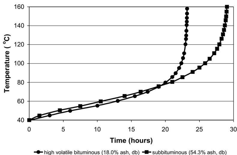
FIG 2 - Adiabatic self-heating curves for coals of approximately the same R<sub>70</sub> value (1.75 and 1.84 C/h).
