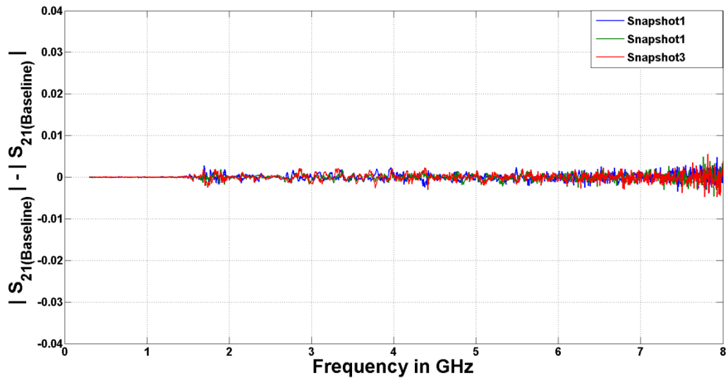
Figure. 3 Three absolute differences between two baseline snapshots superimposed on each other showing the same shape with small variation for each snapshot for 160mm PVC pipe.
