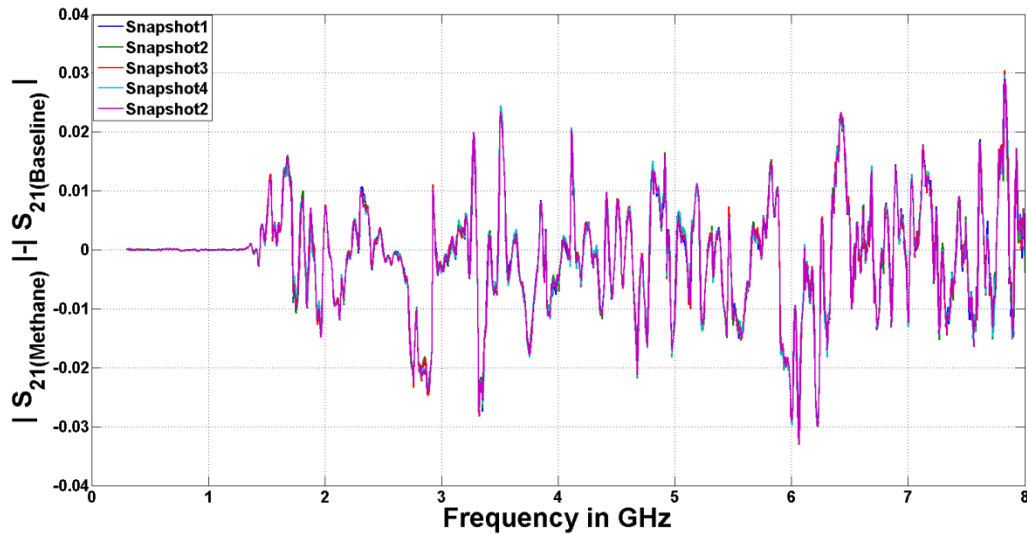
Figure. 6 Five absolute differences between methane and baseline trends superimposed on each other showing the same shape with small variation for each snapshot for 160mm PVC pipe.
