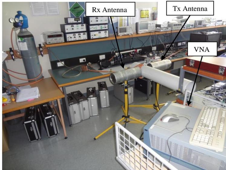
Figure. 1. Experimental setup with 160mm PVC pipe and two turns of the rubber tubing.
